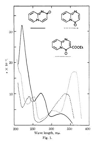
of the product since it is not certain in which of these reactions rearrangement occurs. To decide between structures XVI and XVII, the ultraviolet spectrum of the compound (Fig. 2) was compared with those of I and XIII (Fig. 1). The similarity of the spectrum to that of XIII establishes its formula as XVII. Thus XV obviously must rearrange when cyclized by the action of sulfuric acid.
